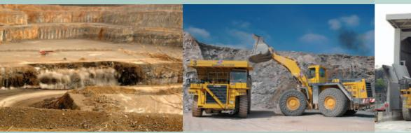
In the quarry, explosives are used to break up limestone or chalk rock. This can dislodge up to 30,000 tonnes of rock in one explosion. The broken rock is picked up at the quarry face by mechanised excavators and loaded into dump trucks or on to conveyors for transportation to the primary crusher. The truck pictured has a payload of over 90 tonnes. Primary crushing of the rock is followed by secondary crushing and screening to separate the rock into a variety of sizes.
